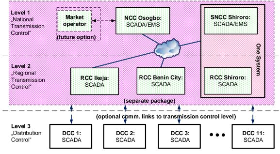
FIGURE 33: OVERALL ARCHITECTURE OF THE DRAFTED SCADA/EMS SOLUTION
