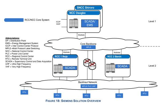
The communication architecture shall be designed in a hierarchical approach. MPLS Technology is used at the fiber optic Core Backbone area and provides high speed IP-data communication for SCADA-, Voice and protection data.
