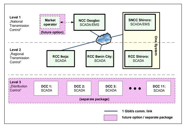
FIGURE 19: OVERALL ARCHITECTURE OF THE DRAFTED SCADA/EMS SOLUTION
