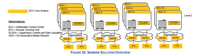
3G/4G public cellular radio technology is used to connect RTUs to the Distribution SCADA systems. With the proposed communication solution, it is possible to use another mobile telecommunication network as a backup in case one telecommunication network is out of service.
